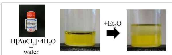
Fig. 3 [AuCl_4]^- was dissolved in both aqueous layer and Et 2 O layer.
