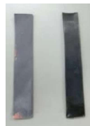
Fig. 15 CuO (left) vs. “ Shakudo -like plating” (right)
