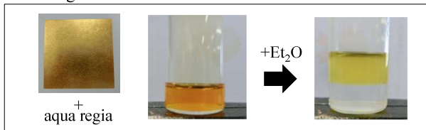
Fig. 2 [AuCl_4]^- was extracted into the Et 2 O layer from the aqueous layer.
