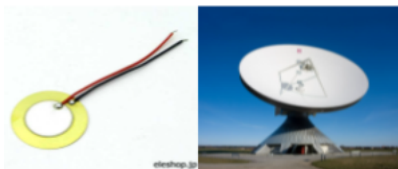
fig.1 piezoelectric element and parabolic reflector.
